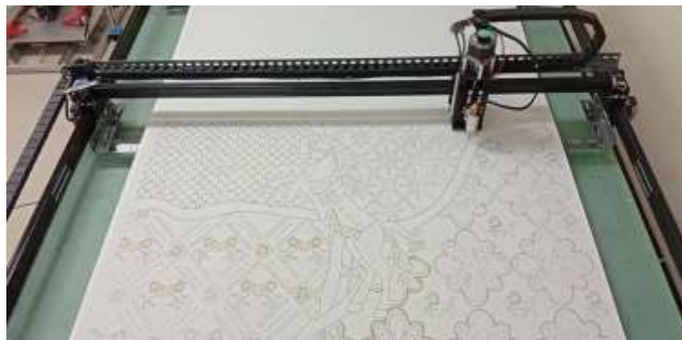
Figure 3. The batik-making process for the Batik Bambu Mujur pattern using Smart Canting.
