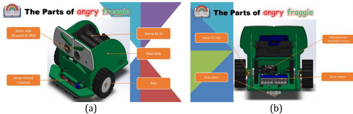
Figure 2. Part of "Angry Froggie" Robot (a) at the front, (b) at the back.
