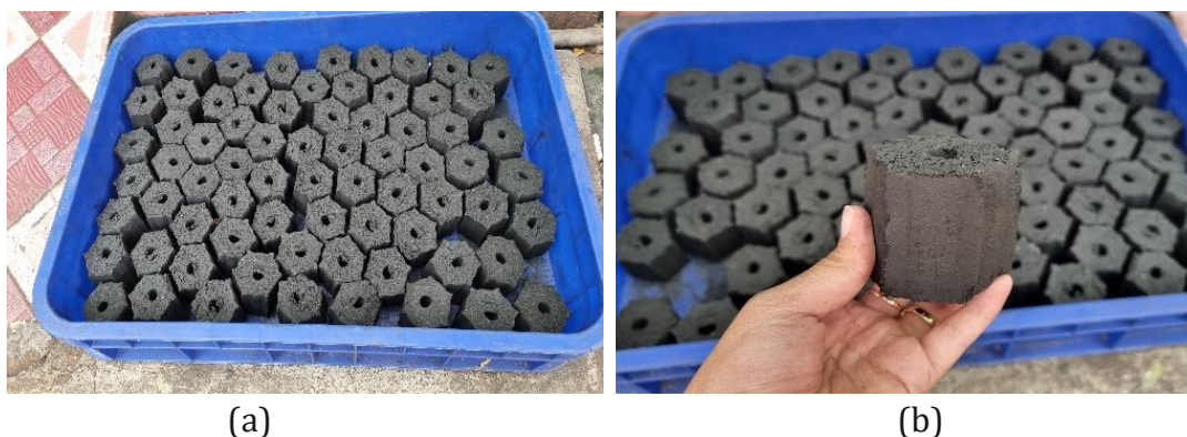
Figure 8 (a), (b). The Results of Charcoal Briquettes Using An Automatic Printing Machine
