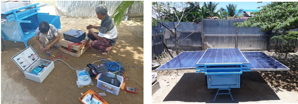
Figure 4. Design and Testing Process of Portable Solar-Powered Submersible Pump Technology
